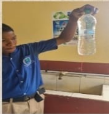
Testing the 1mm in diameter hole at the bottom of the 1 litre bottle.
